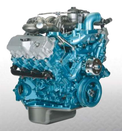
The parent bore International VT 275 features a rating of 200 hp (149 kW) and 440 lb-ft (597 N•m) of torque.
